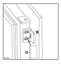
After completion of the door reversing operation, check that the door gasket adheres to the cabinet. If the ambient temperature is cold (i.e. in Winter), the gasket may not fit perfectly to the cabinet. In that case, wait for the natural fitting of the gasket or accelerate this process by heating up the part involved with a normal hairdryer on a low setting.
